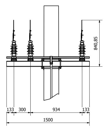
Dimensions of load break switch RN
