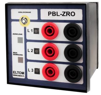
connected to the output of the measuring insulators. Switching relay: authorization is only in the absence of currents in the input circuits (currents below the threshold) and after pushing the 'odblokowanie button' for about 30 sec. Input circuit clamps are located on the rear panel. For proper operation of the relay you need auxiliary power supply to be connected to the clamps on the rear panel (L +, N-).
